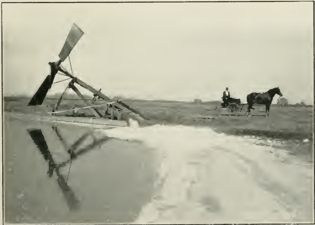
ARCHIMEDES SCREW WINDMILL—ALAMEDA SALT WORKS. USED FOR PUMPING BRINE FROM THE TANKS
